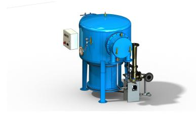
From this reservoir the distillate is drawn out of the separator by a freshwater pump which sends along distillate through the salinity sensor and the water meter. In case of too high salinity the sensor will by-pass the distillates up into the separator again by activating a solenoid valve. The salinity can be read on the salinometer.
